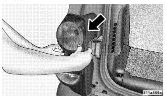
3. Unlock and remove electrical connector.
